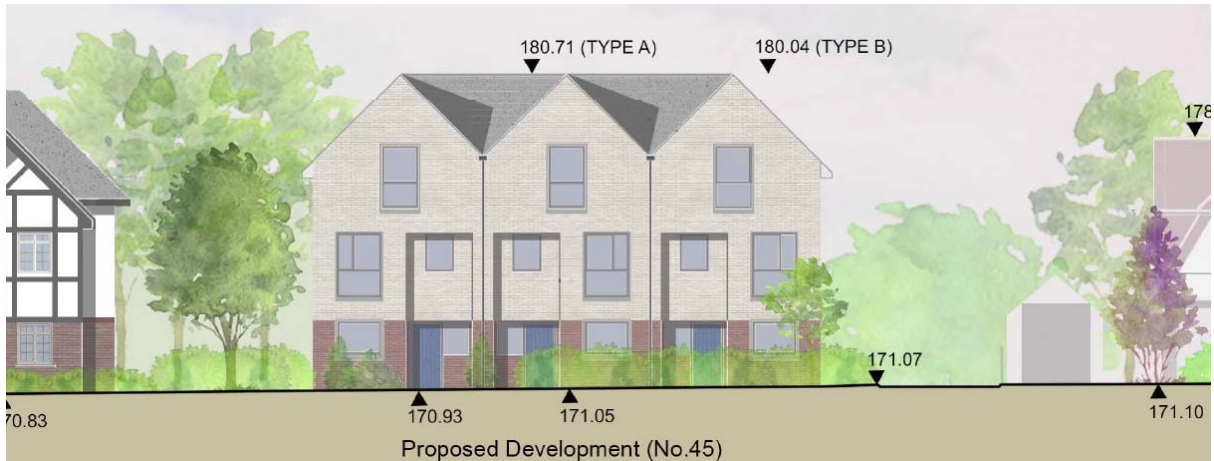
Fig 3: Elevational view highlighting the front of the proposal in relation to neighbouring properties.
